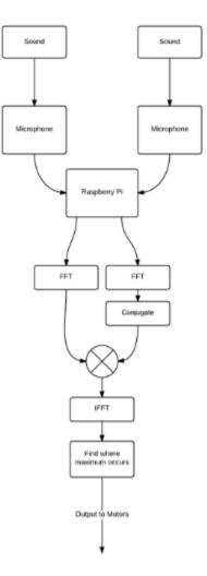
Fig. 14. Determining Time Delay Between Similar Sounds
