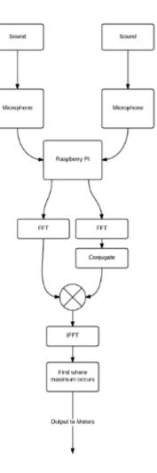
Fig. 9. Determining Time Delay Between Similar Sounds
