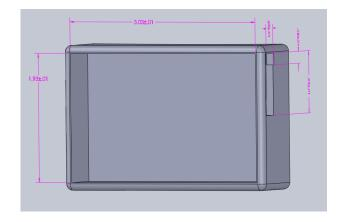
Fig. 7. CAD Design for Headphone Attachment
