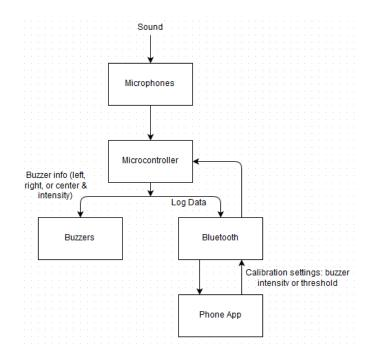
Fig. 15. High-level Block Diagram of the Sonic-Vibe
